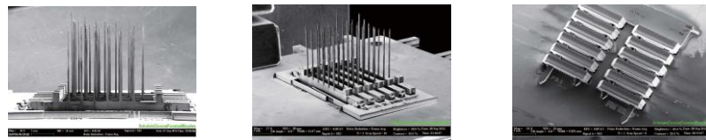
Above, left and center: Assembled 3-D array, demonstrating the construction mechanisms. The above array has 40 needles, with three electrode sites along every needle. Each needle was customized, and in this example designed with a unique length and placed at varying positions along each 2-D insert. The V-shaped alignment bracket mechanism is seen in the center. Right: underside of the 3-D array showing the self-locking assembly mechanism, as well as the electrical connections between the base plate and each array insert.
