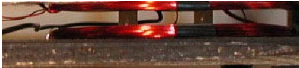
Figure 5: Spacing between the 10-turn and 38-turn coils
