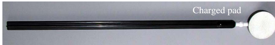
Figure 4 One of two charge producers (the other has a blue charged pad)
