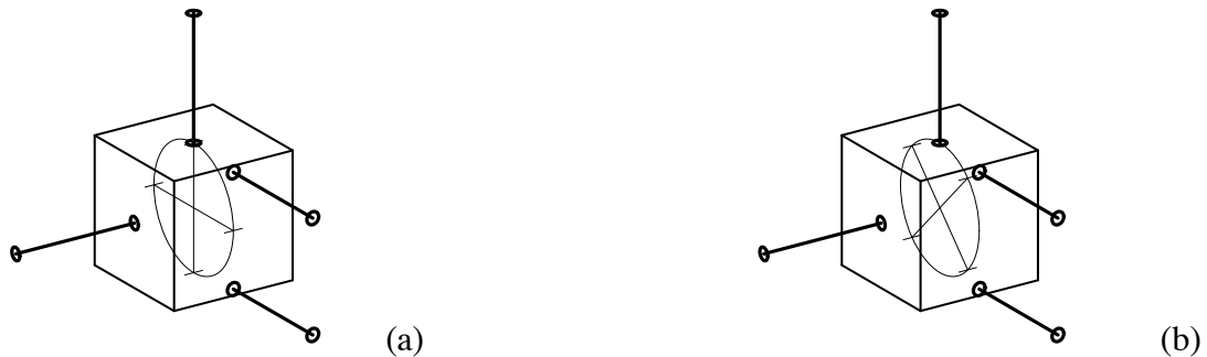
Figure 2-24 The circle lies in the plane of three constraints and the fourth constraint intersects its center. Any distinct pair of rotational axes that lie in this plane and intersect the center will represent the instantaneous motions allowed by the constraints.
