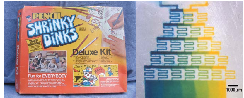
Inkjet printed microfluidics in Shrinky Dinks (polystyrene) and Silicone rubber
