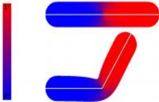
Figure 8: Top: heat equilibrium for two bones. Bottom: the result of rotating the right bone with the heat-based attachment
