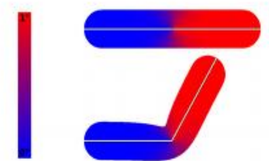
Figure 8: Top: heat equilibrium for two bones. Bottom: the result of rotating the right bone with the heat-based attachment
