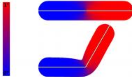
Figure 8: Top: heat equilibrium for two bones. Bottom: the result of rotating the right bone with the heat-based attachment
