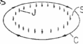
Figure 9.4.2 Surface S enclosed by contour C used with Ampère's integral law to determine \mathbf{H} in the coil shown in Figure 9.4.1.
