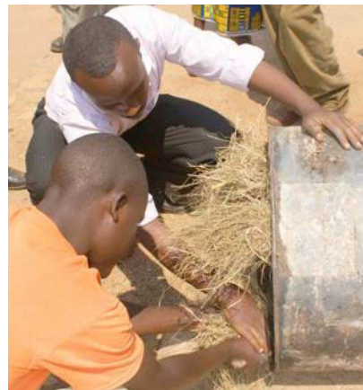
Figure 8: Make 'wicks' in the bottom of the oil drum Photo credit: Fuel from the Fields
