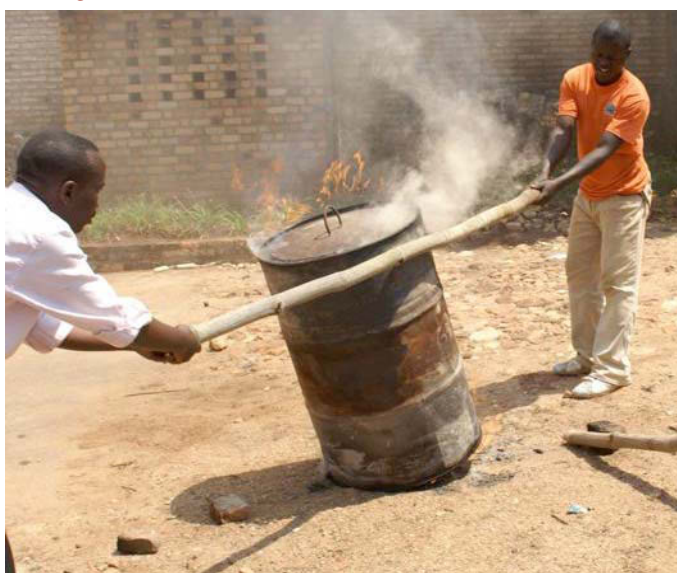
Figure 13. Gently lower the drum to seal off the air holes on the bottom. Photo credit: Fuel from the Fields
