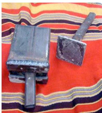
Figure 3: A briquette press, made from angle iron and sheet metal. Photo credit: Fuel from the Fields
