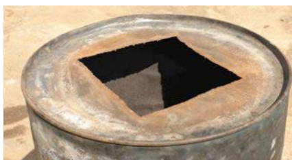
Figure 4: The square loading hole in the top of the drum. Photo credit: Fuel from the Fields
