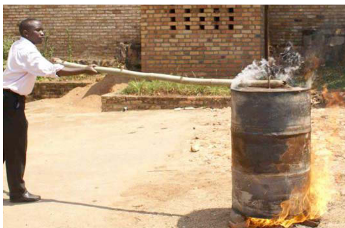
Figure 12. Place the lid on the drum Photo credit: Fuel from the Fields
