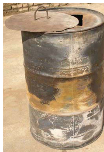
Figure 2: A steel oil drum with lid forms the kiln. Photo credit: Fuel from the Fields
