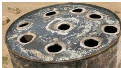
Figure 5: 9 small air holes in the bottom of the drum. Photo credit: Fuel from the Fields
