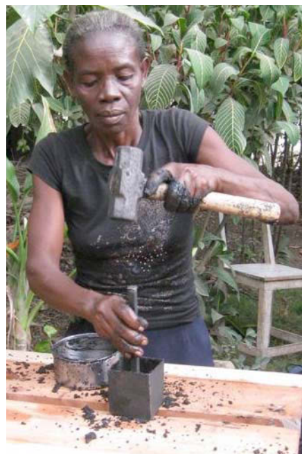
Figure 16. Using the briquette press Photo credit: Fuel from the Fields
