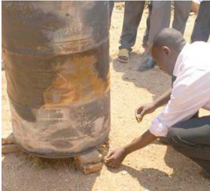
Figure 9: Raise the drum on three flat stones, and light the wicks at the bottom. Photo credit: Fuel from the Fields
