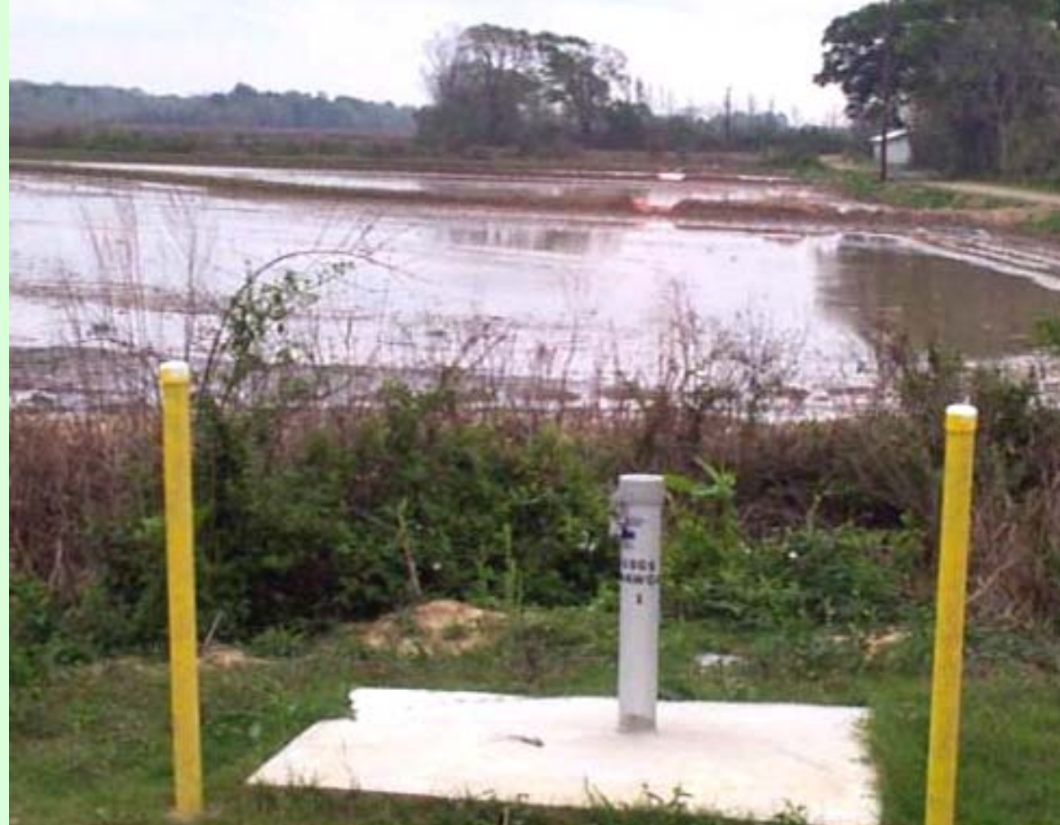
“Stick-up” well and protective cover
