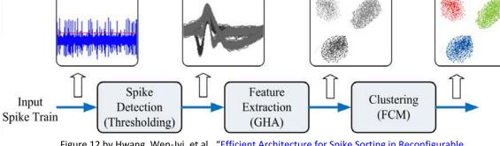
Figure 12 by Hwang, Wen-Jyi, et al., "Efficient Architecture for Spike Sorting in Reconfigurable Hardware." Sensors 13 no. 11 (2013): 14860-14887. MDPI Open Access. License: CC BY.
