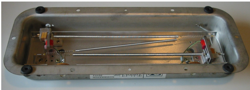
Figure: O. C. Electronics Folded Line spring reverb (© Unknown. All rights reserved. This content is excluded from our Creative Commons license. For more information, see http://ocw.mit.edu/help/faq-fair-use/ )
