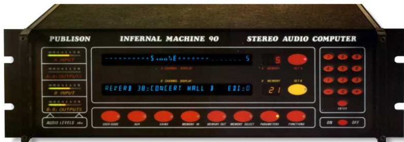
Figure: Publison Infernal Machine 90 digital audio processor (ca. 1987) (© Unknown. All rights reserved. This content is excluded from our Creative Commons license. For more information, see http://ocw.mit.edu/help/faq-fair-use/ )
