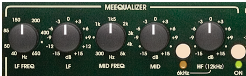
Figure: EQ section of a Joemeek twinQ microphone preamp (© Joemeek. With edits. All rights reserved. This content is excluded from our Creative Commons license. For more information, see http://ocw.mit.edu/help/faq-fair-use/ )
