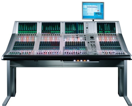
Figure: Studer Vista digital mixing console (© Studer Professional Audio GmbH. All rights reserved. This content is excluded from our Creative Commons license. For more information, see http://ocw.mit.edu/help/faq-fair-use/ )
